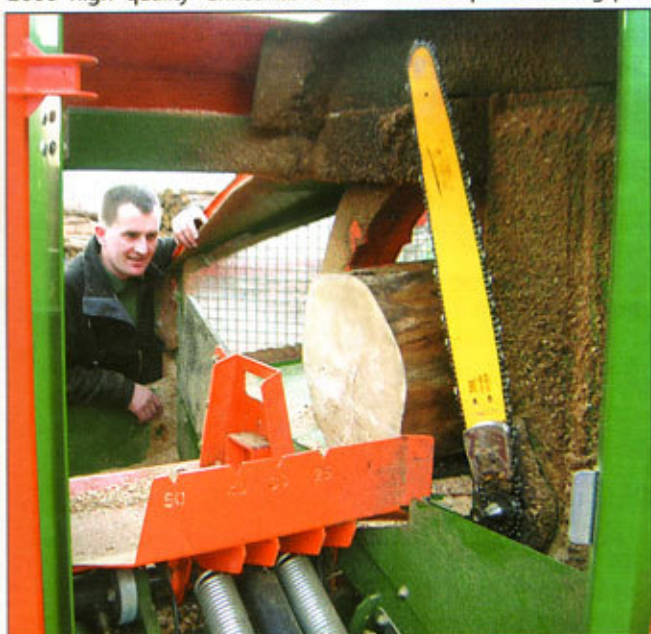
(Left) Chainsaw crosscut fitted with hardened harvester chain, capable of cutting 18 inch material. (Right) Melanie Burman is just visible as she fills the Marshall trailer.
