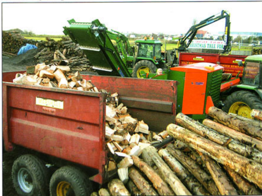
(Left) Chainsaw crosscut fitted with hardened harvester chain, capable of cutting 18 inch material. (Right) Melanie Burman is just visible as she fills the Marshall trailer.
