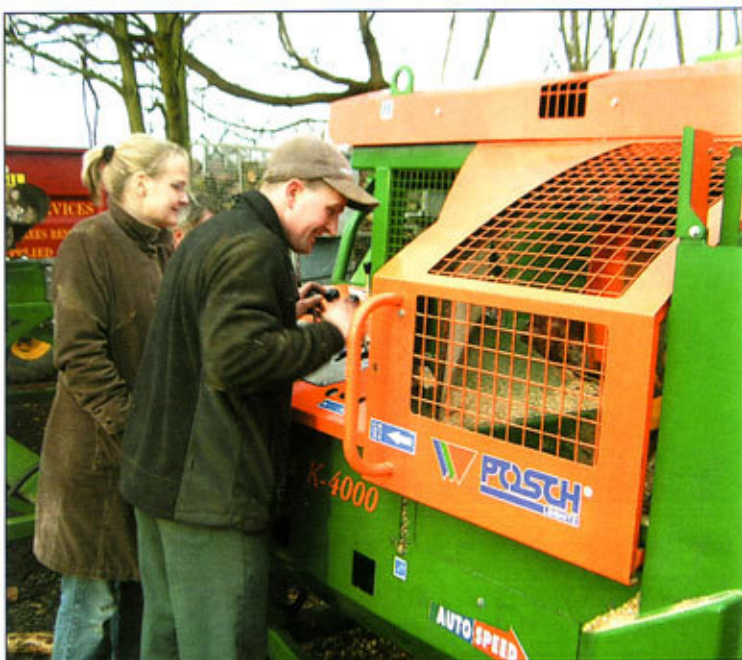
Andrew and Melanie Burman with their new Posch K-4000. The controls are offset allowing the operator to view the cutting process through a perspex screen which protects him from sawdust and flying debris.
